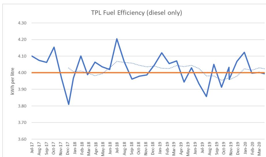
**Figure 16: Diesel efficiency performance of TPL. Computed using TPL data.**
